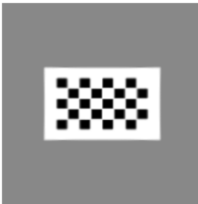
Figure 1-5: The distorted image corrected with coefficients (-10, -100, -1000) for the radial distortion correction equation applied.
